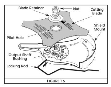
4. Make sure that the cutting blade is centered on the pilot step and sitting flat against the output shaft bushing. See Figure 17.
